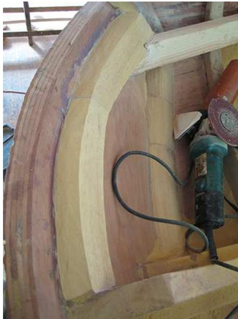
FIG.7. The picture shows a wooden boat in the making at the Michelsen boatyard in D-Friedrichshafen in 2010. The angle grinder seen in the picture is used to "carve" the complex compound curves of the transom frame on the left.
