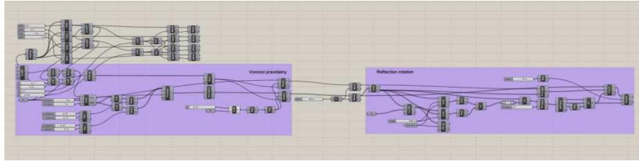
FIG.16: Grasshopper plug-in for Rhinoceros is calculating angles of mirror tilts. (graphic: Michal Kotvan)
