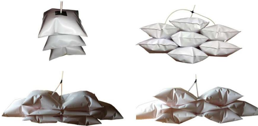
FIG.9: Various positions of inflatable parts of the wall during the prototyping process. (photos: Dominika Szabová)
