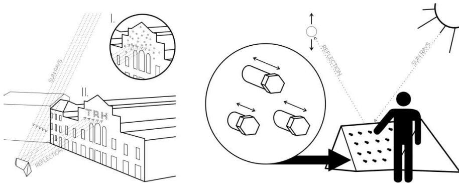
FIG.17: Sunlight reflector principles. (graphic: Michal Kotvan)
