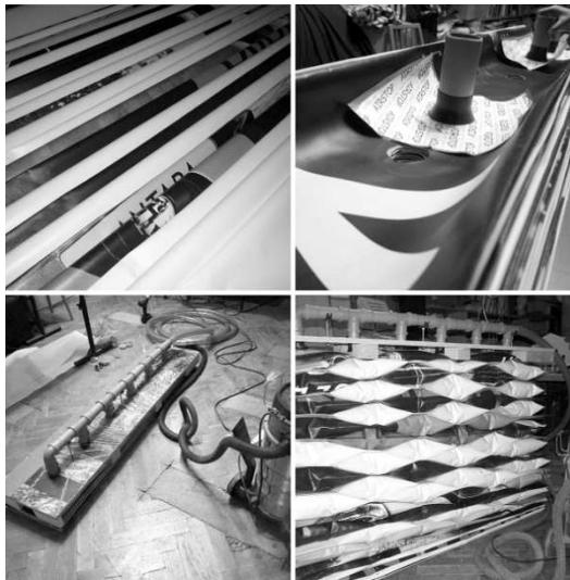
FIG.8: Process of final prototype constructing: cutting and linking banners – connecting with source of inflating – preparation of supporting structure – inflating the prototype. (photos: Dominika Szabová)
