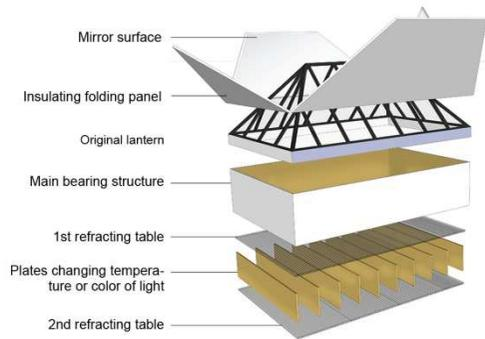
FIG.7: Construction parts of skylight. (schema: Lucia Trangošová)
