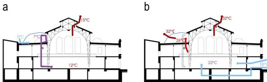
FIG.3: Energy buffer zone concept: a – obtaining solar energy for heating in winter, b – cooling in summer (schemes: Katarína Šoltýsová)
