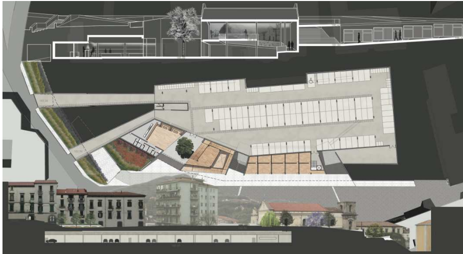
FIG.3 Project for San Francisco Square. Plan of the underground level, sections along the in-between spaces (above) and the parking (below).
