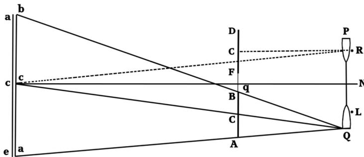
Figure 17 – Diagram for Sutton's (1856b) Theory of the Stereoscope. P and Q are semi-lenses. DCF and BCA are images on the stereogram. ace (mislabeled: it should be dcf) and bca are virtual images. Sutton makes the common mistake of assuming that all points on the stereogram will be "measured" at the same angle of convergence (RcQ).
