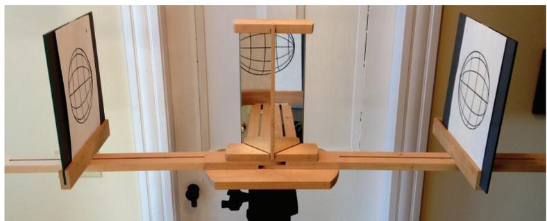
Figure 1 – *Wheatstone Stereoscope*. This is a replica of Wheatstone’s 1852 design with adjustable image plates (to change the size of the retinal images projected) and moveable arms that allowed adjustments to the (base) angle of convergence of the eyes.
