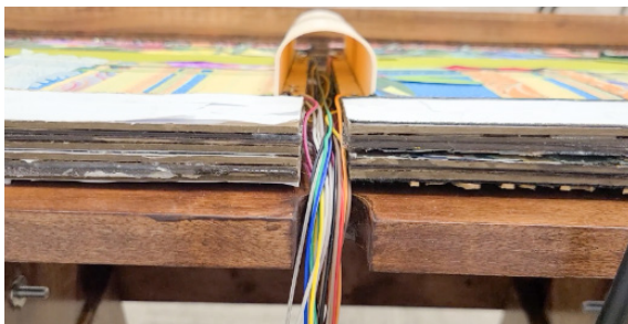
Figure 13 Makey Makey wires running to the edge of the page, into the hollow spine, and behind the podium. Early prototype from first beta playtest.
