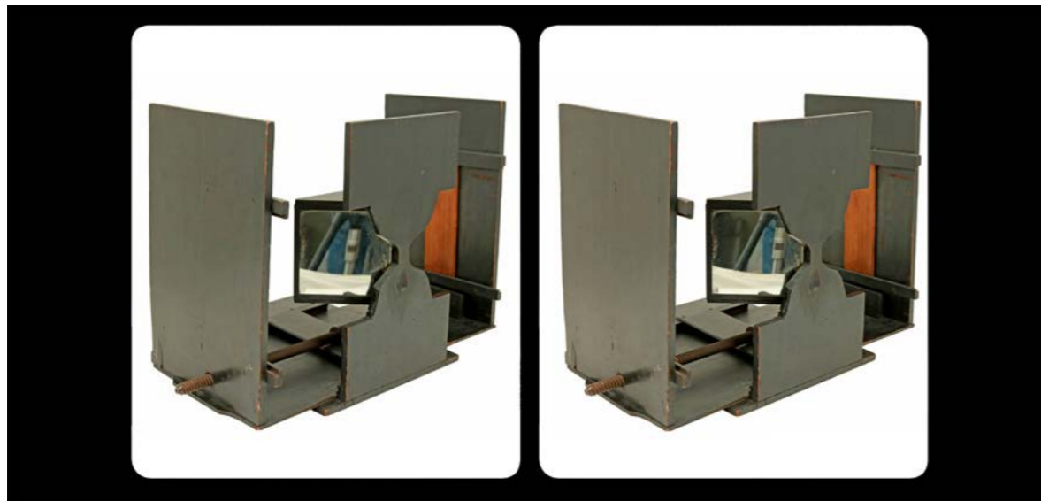
Figure 1. Wheatstone’s original 1838 stereoscope, now in the Science Museum, London.
