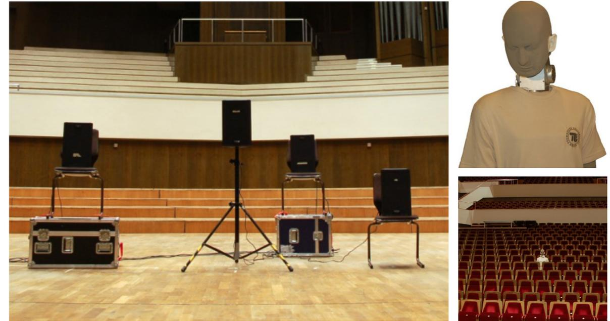
Figure 3: Playback of excitation signals and recording of binaural room impulse responses using the head and torso simulator *FABIAN*.
