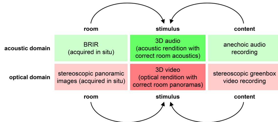
Figure 1: Technical concept. The simulation requires a mutual independence of 1<sup>st</sup> the acoustical and the optical domain, and 2<sup>nd</sup> the room and the artistic performance.
