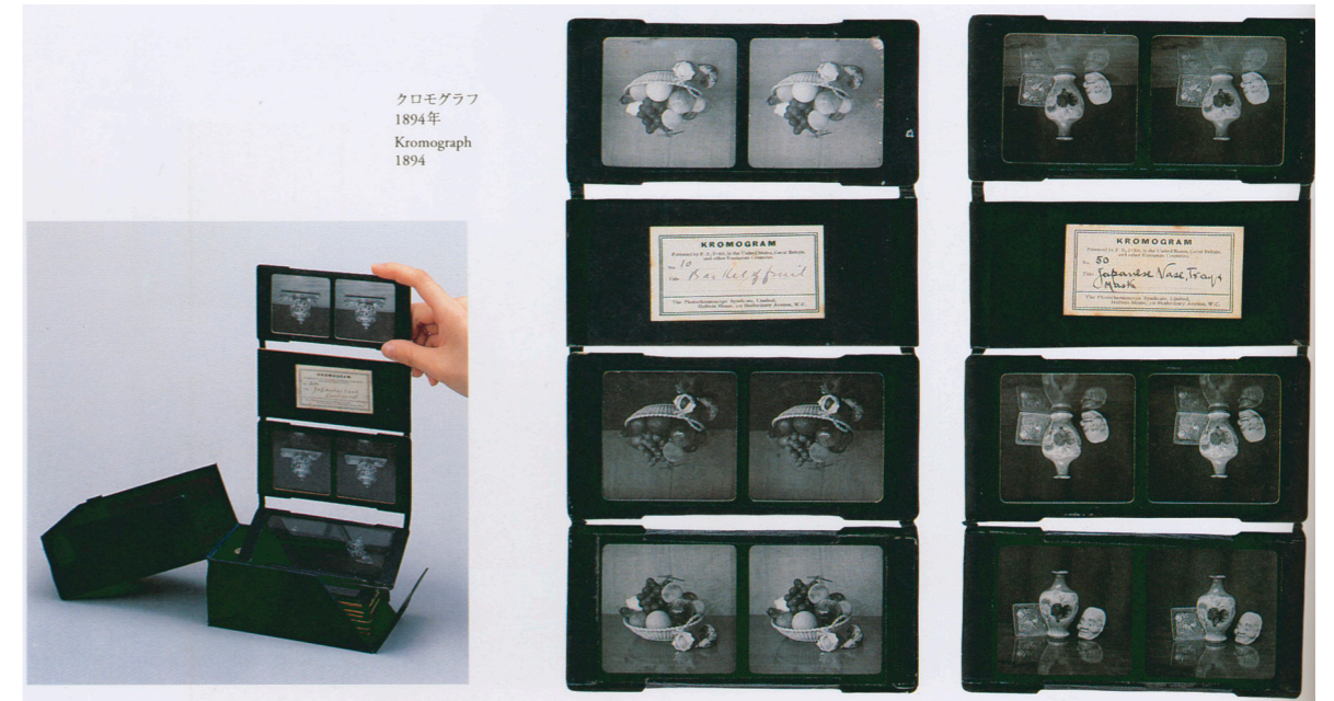
Fig.4 Kromographs by F. Ives, three linked sets of stereo pairs, taken through three different colour filters, within the Kromskop ; a system of prisms combined all three.
