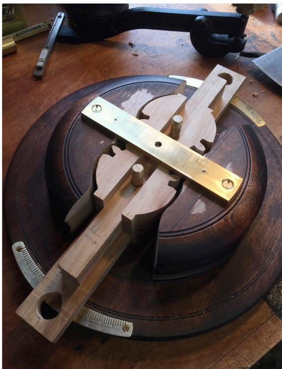
**Fig. 14** Stereoscope Gears. These gears will synchronise the motion of the arms of the stereoscope, which have yet to be attached. Unlike Wheatstone's design (Fig. 13) there are two pivots here spaced at about the inter-ocular distance, so the angular measures more accurately reflect what is happening to the eyes.
