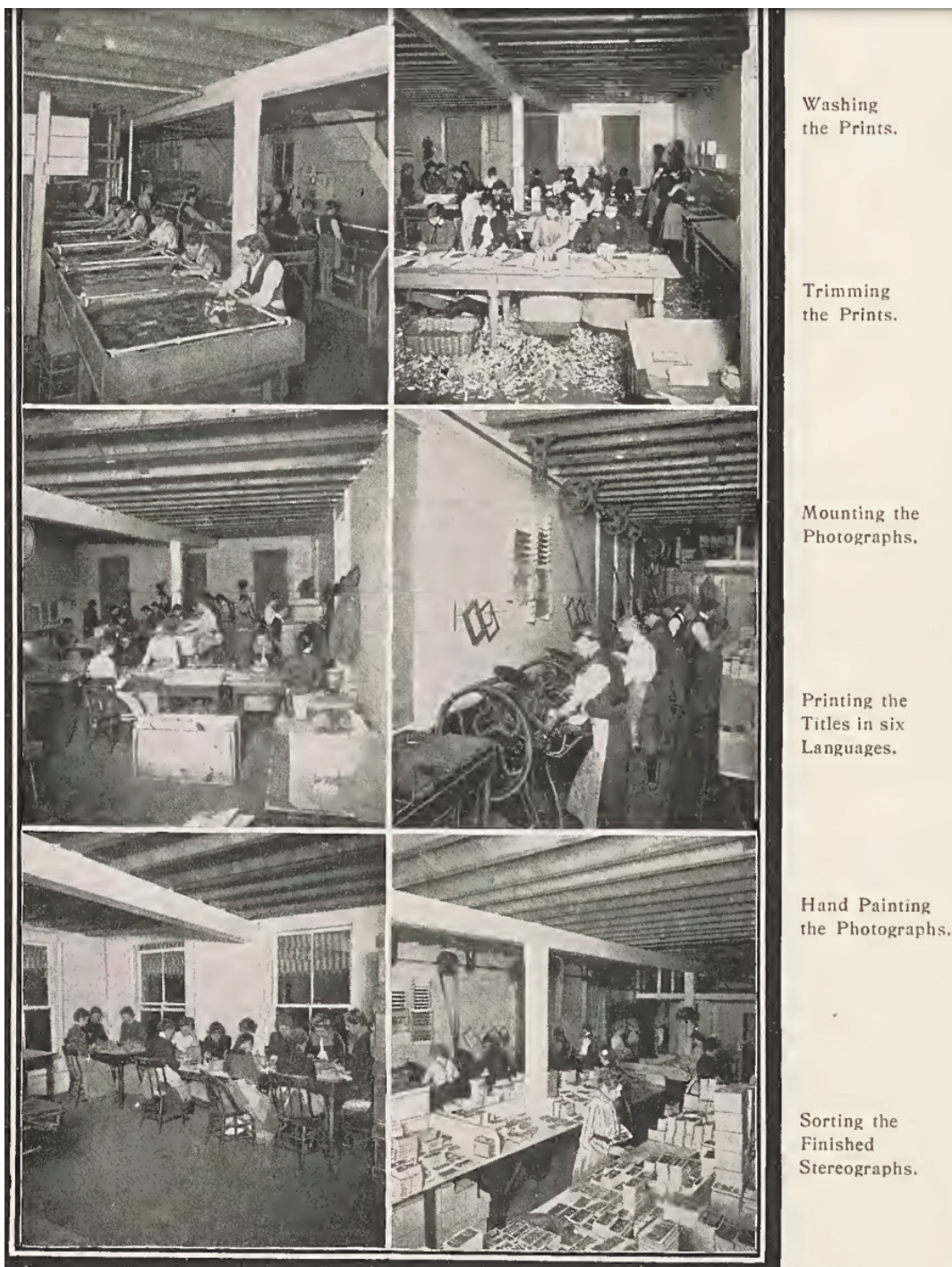
Fig. 2 Images of the stereograph production line, from The Stereoscopic Photograph. Courtesy Smithsonian Libraries and Archive.
